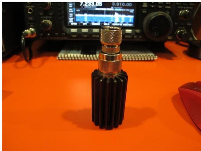
you're using an antenna analyzer. You put this little guy in your pocket and take it up on the roof, or tower. You don't need a high power load for the analyzer so the small load is perfect for what you're doing. These are also great if you are tuning a filter circuit or a set of duplexers. Very handy to have a little guy.
